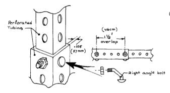
fig. 2. Right angle bolts connect tubing sections.
